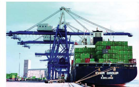
40.5t Quayside Container Crane
