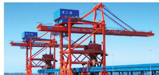
2250t/h Ship Unloader in Zhanjiang Port
