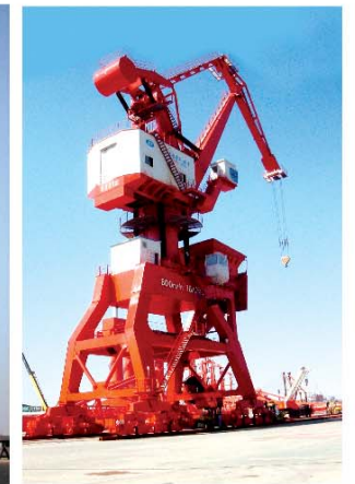
800 t/lb Portal Crane
